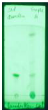
Figure 5: Comparison of TLC profile of Quercetin (left side) and ethylacetate fraction (right side) of methanol extract
