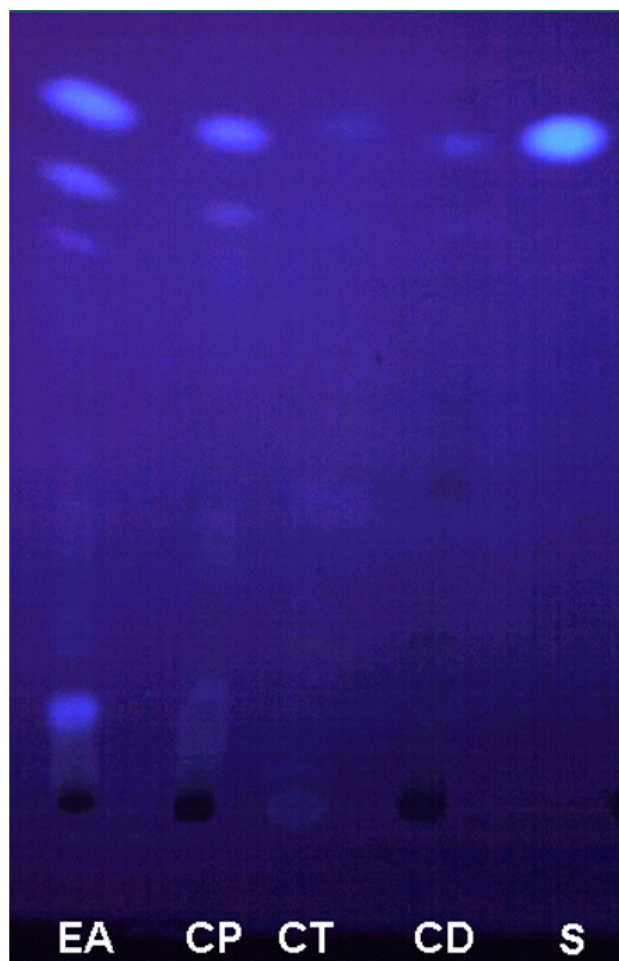
Fig. 1: Comparatives TLC of ethanolic extracts of CD, CT, EA and CP with scopoletin (S) ( R_f = 0.81 in UV 366 nm.)
