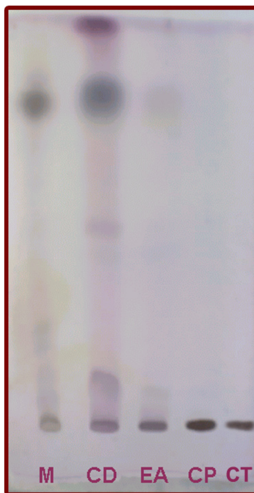
Fig. 2: Comparatives TLC of ethanolic extracts of CD, CT, EA and CP with mangiferin (M) ( R_f: 0.72 with 1% FeCl_3 sol.)
