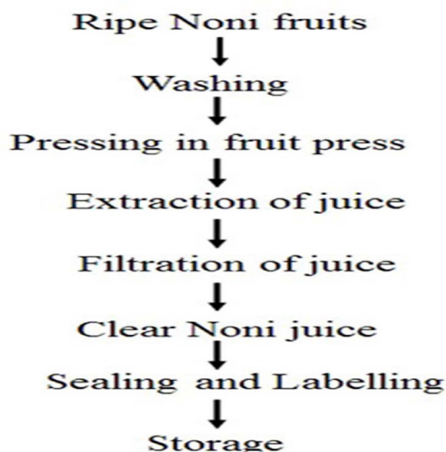
Figure 12: Flow sheet for production of Non-traditional Noni juice.
