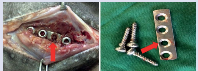
Figure 3: Physical examination of the plate macroscopically in the 304 stainless-steel plate group. The arrows indicate no change in muscle and plate discoloration after implantation.
